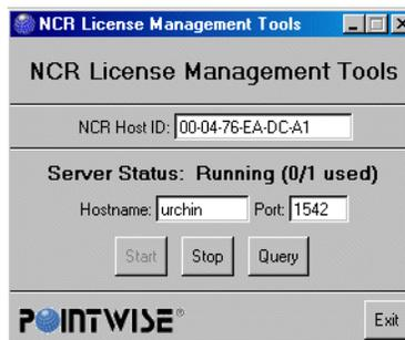
4. Press the **Query** button to show the number of NCR processes being used and the number of NCR processes that are available for the current NCR license file.
