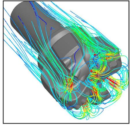
Pointwise was used for the mesh, left, in this drill bit simulation. ANSYS® FLUENT®, center, and OpenFOAM® were used for the flow.
