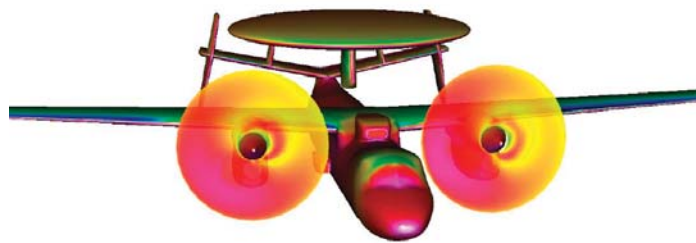
E-2C prop blade element model including swirl.
